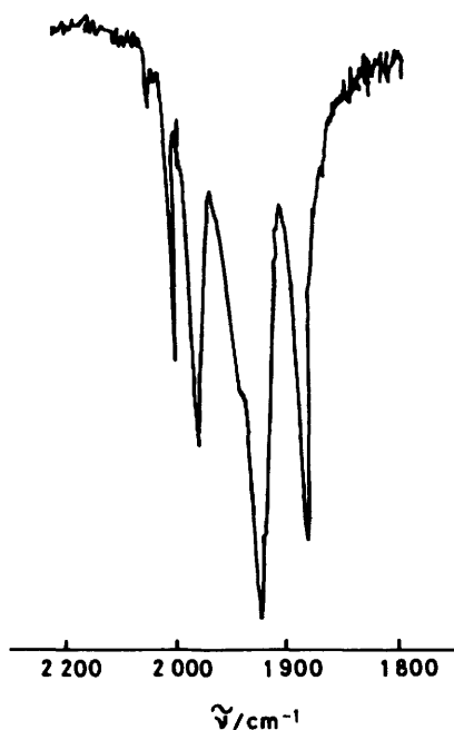
Figure 1. I.r. spectrum in the \nu(\text{CO}) region of the hypothetical trianion derived from (1a) and NaH in thf in the presence of ethanol
